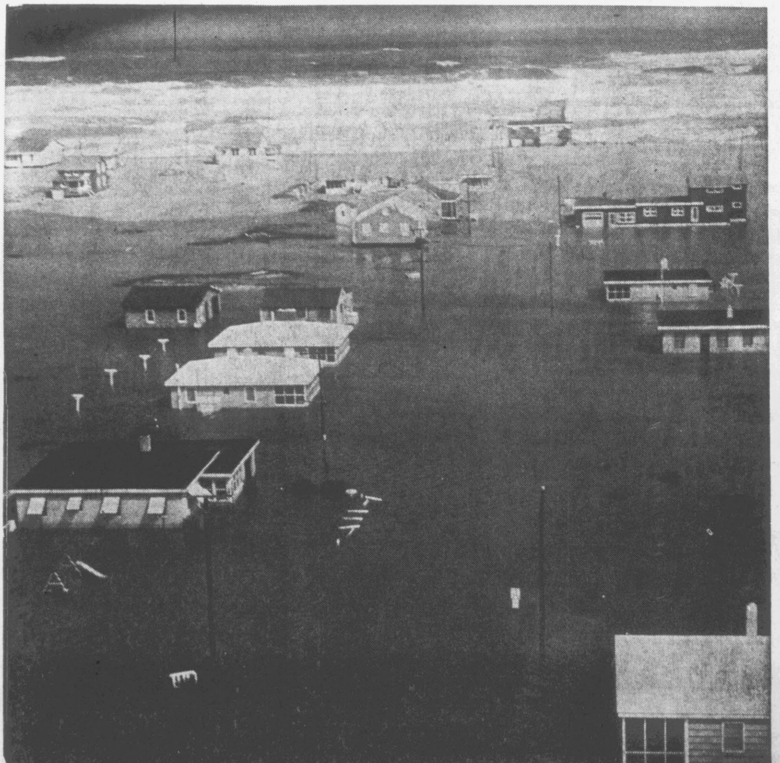
BARRIER DUNES . . . once held out waters of the Atlantic Ocean but now, with dunes eaten away by raging surf, water spills over into area between ocean and the beach bypass road, flooding homes and businesses. Note fishing pier at end of flooded street, with part of its wooden walkway torn away.
