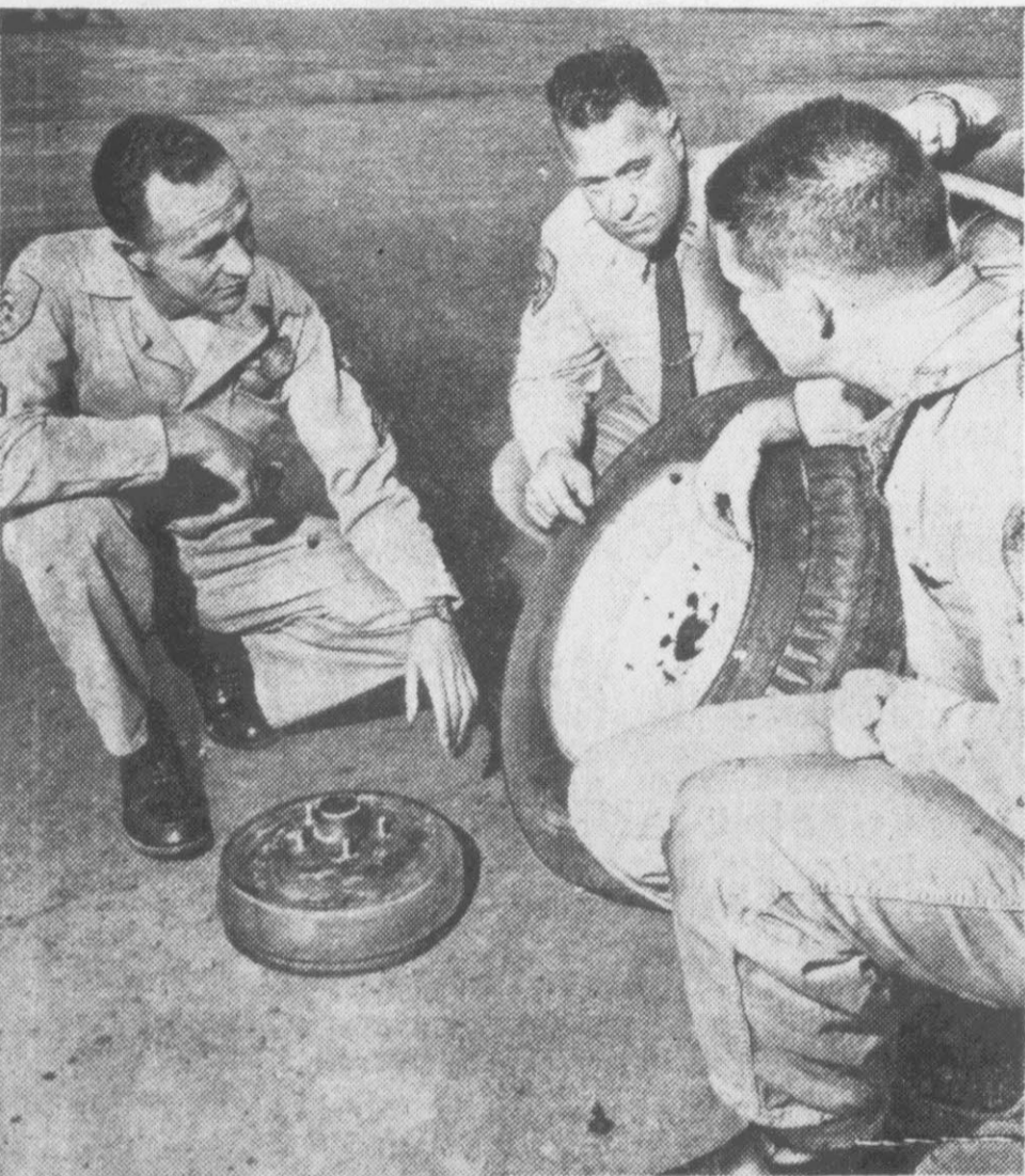
Wheel and drum casualties of academy's high speed track are examined by Sgt. Robert Phillips, left, Capt. Leonard Overhouse, center, commander of academy, and Cadet Verby Pierce. Even with reinforced wheel drums and wheels, parts crack under strain of hard driving.
