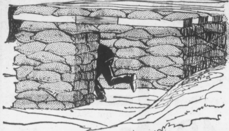
An offset protects shelter from fallout rays.
