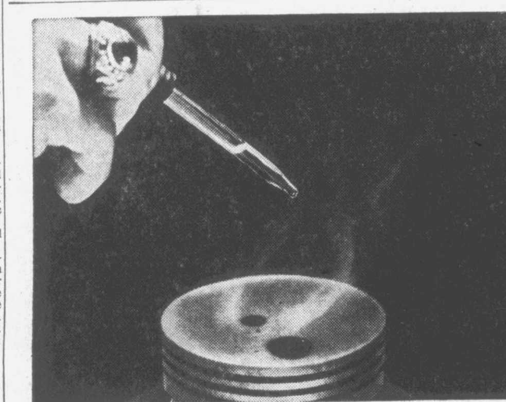
Ordinary oils can create their own metallic ash. Above you see what happens when a conventional multi-grade oil is dropped on this electrically heated piston device. These dark spots contain additive ash. When this ash builds up in your engine, it's bad news.
