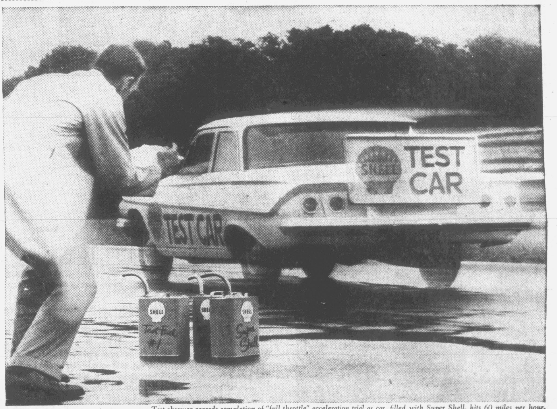
Test observer records completion of "full throttle" acceleration trial as car, filled with Super Shell, hits 60 miles per hour.
