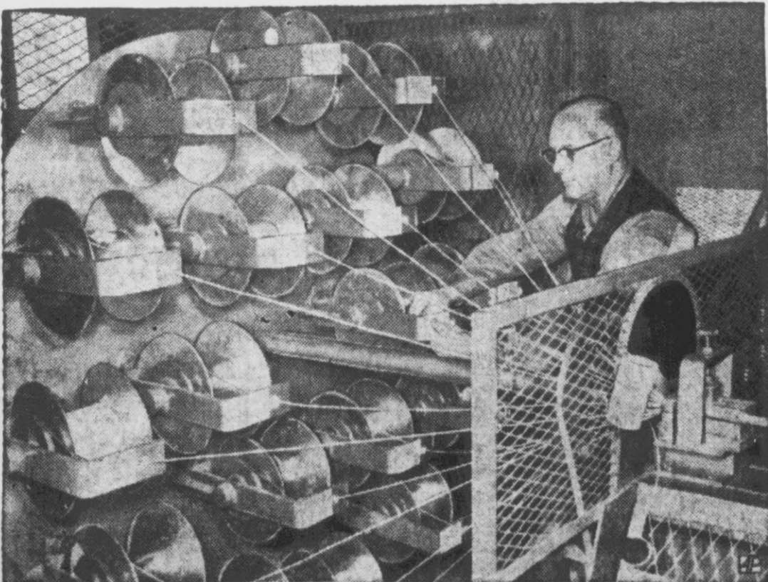
SPACE AGE SPINNER—Technician Arthur Harris checks one of the 18 spools on six-foot diameter wheel of a planetary wire-stranding machine at Van Nuys, Calif. Machine turns out multi-wired cables used for missile and satellite electronic operations.
