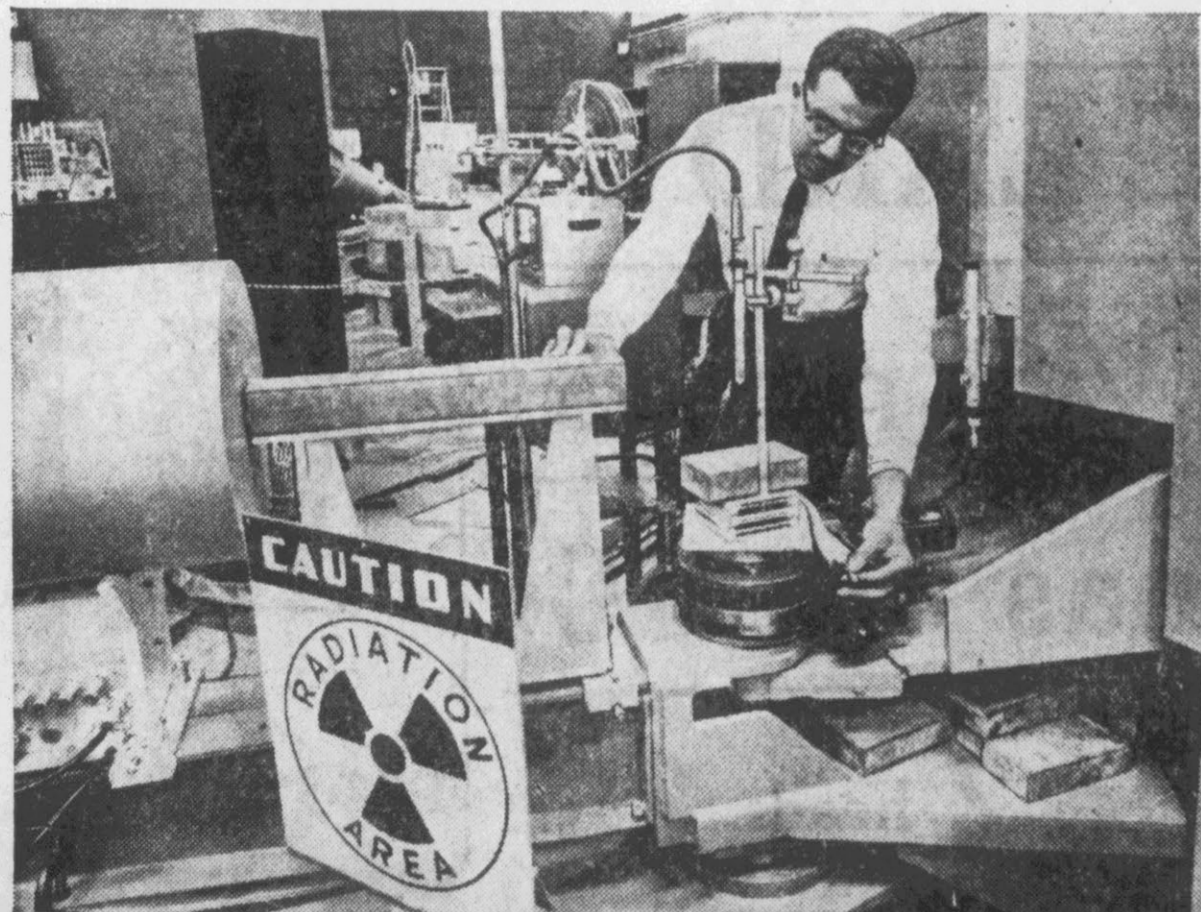
Physicist uses diffraction spectrometer in study of magnetic structure of manganese fluoride.
