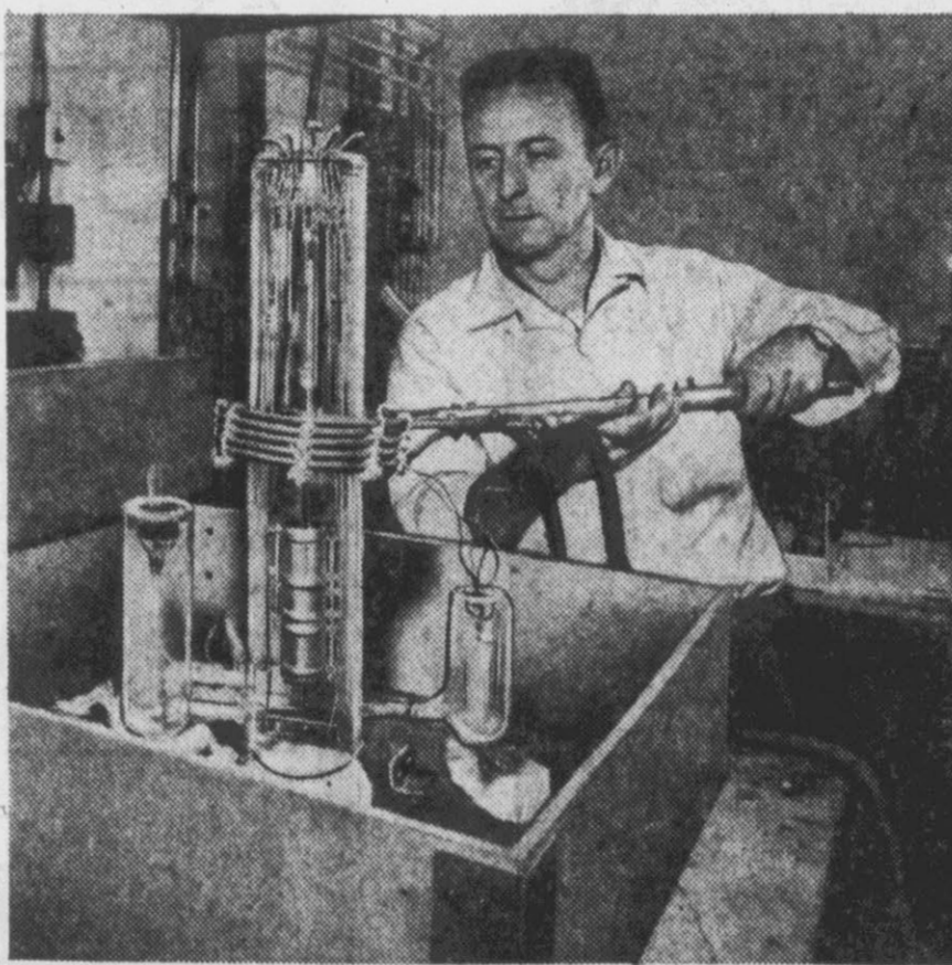
Technician processes cathode tube designed for electron emission studies. Tube is in final stages of cooling after having been baked in oven. It will be used in vacuum tube studies.
