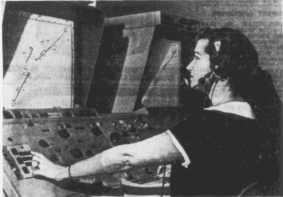
Aircraft simulator, with operator Mrs. Margaret Madsen at controls. Position of simulated aircraft appears as moving dot of light on screen.
