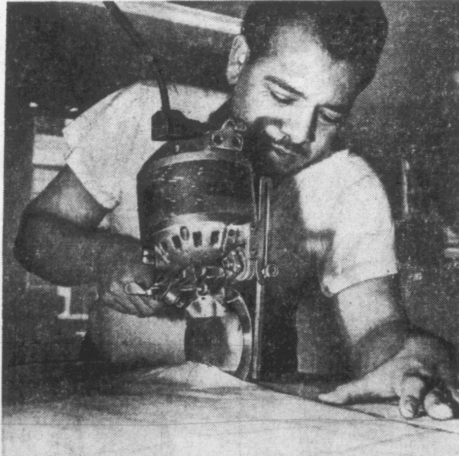
3. Power cutter slices through layers of fabric, topped by white paper on which pattern has been drawn, as cutter does his job.
