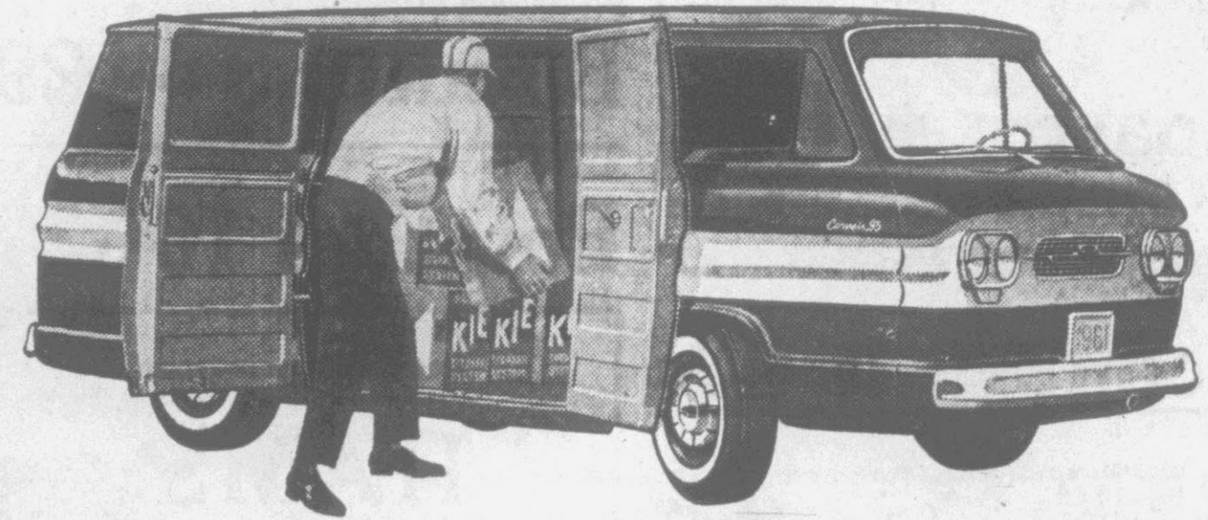
CORVAN—Side doors open a full 49" wide. Loading height is a low 14" HRI!
