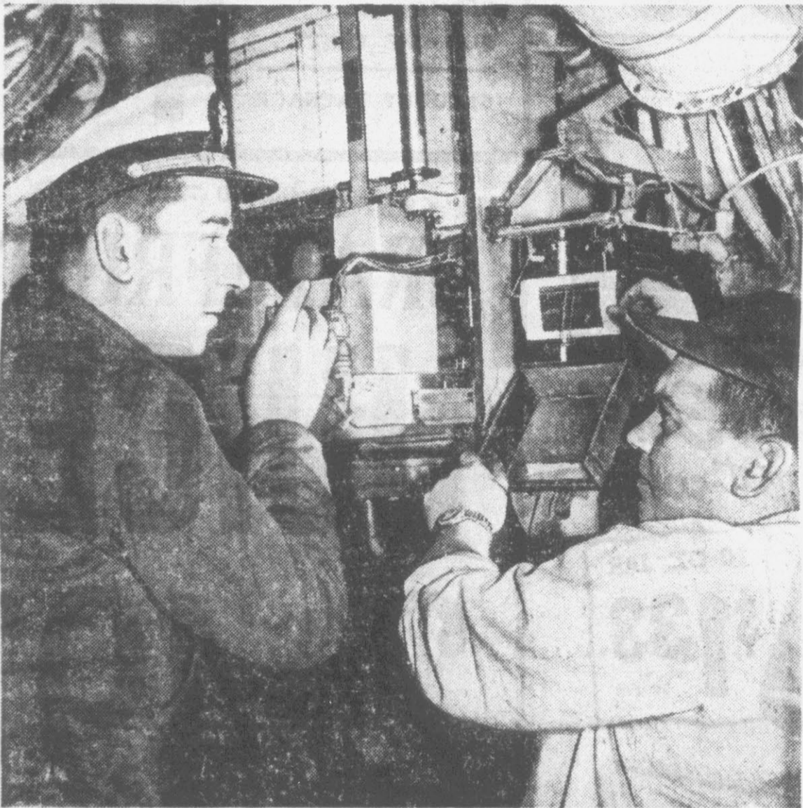
Ship's executive officer, Lt. David Dimmick, left, looks over recording depth gauge in control room, as Alvin Williams, IC 1 (SS), checks bathythermograph, a gadget which combines recording of ship's depth and temperature of water.
