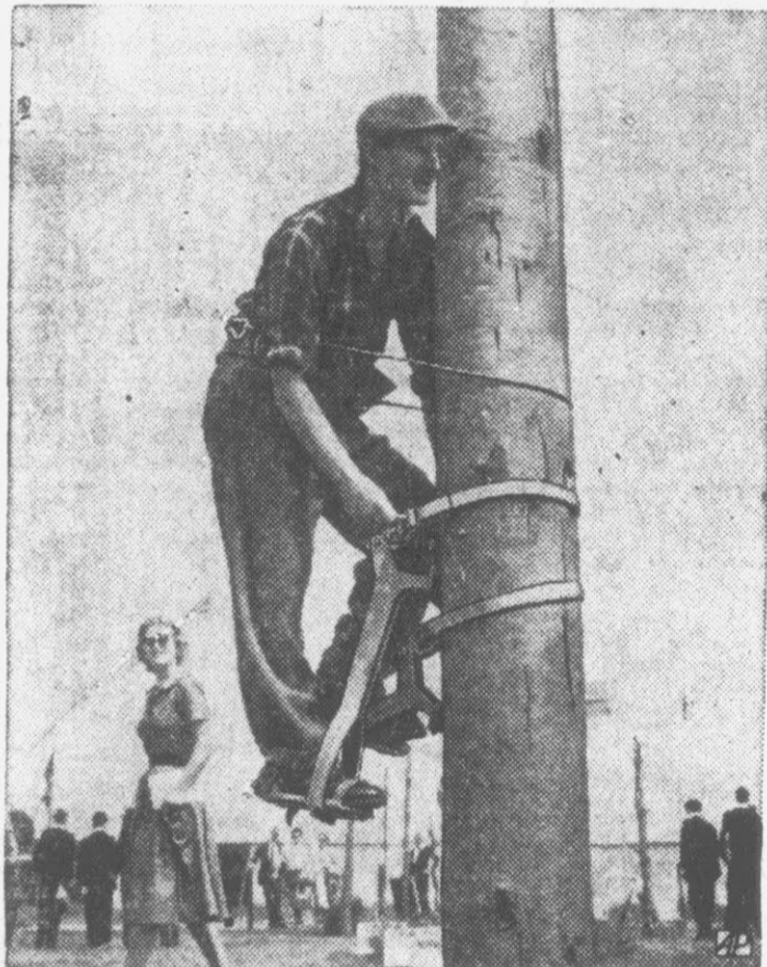
UP BY DEGREES — A forester demonstrates a tree climber at agricultural show in Bath, Eng. The Swiss invention uses grips and pedals to facilitate ascent.
