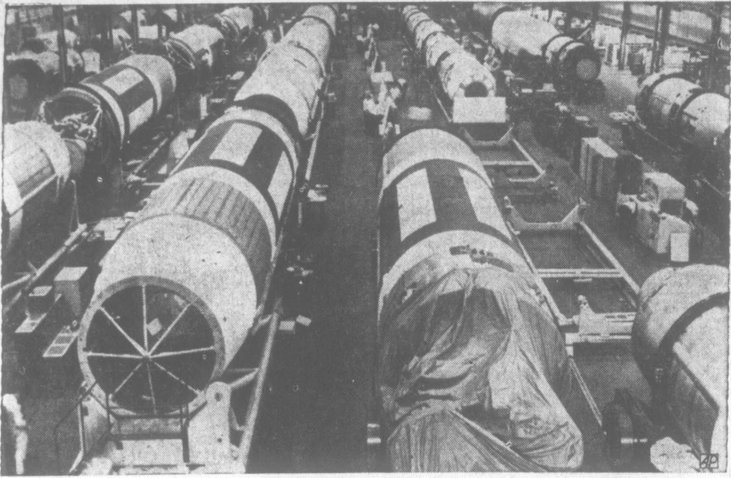
SETTING THE STAGES—First and second stages of the Air Force's Titan ICBM are on the assembly line in a Denver plant. A completed first stage is shrouded, foreground, ready for transport to the Cape Canaveral, Fla., area.
