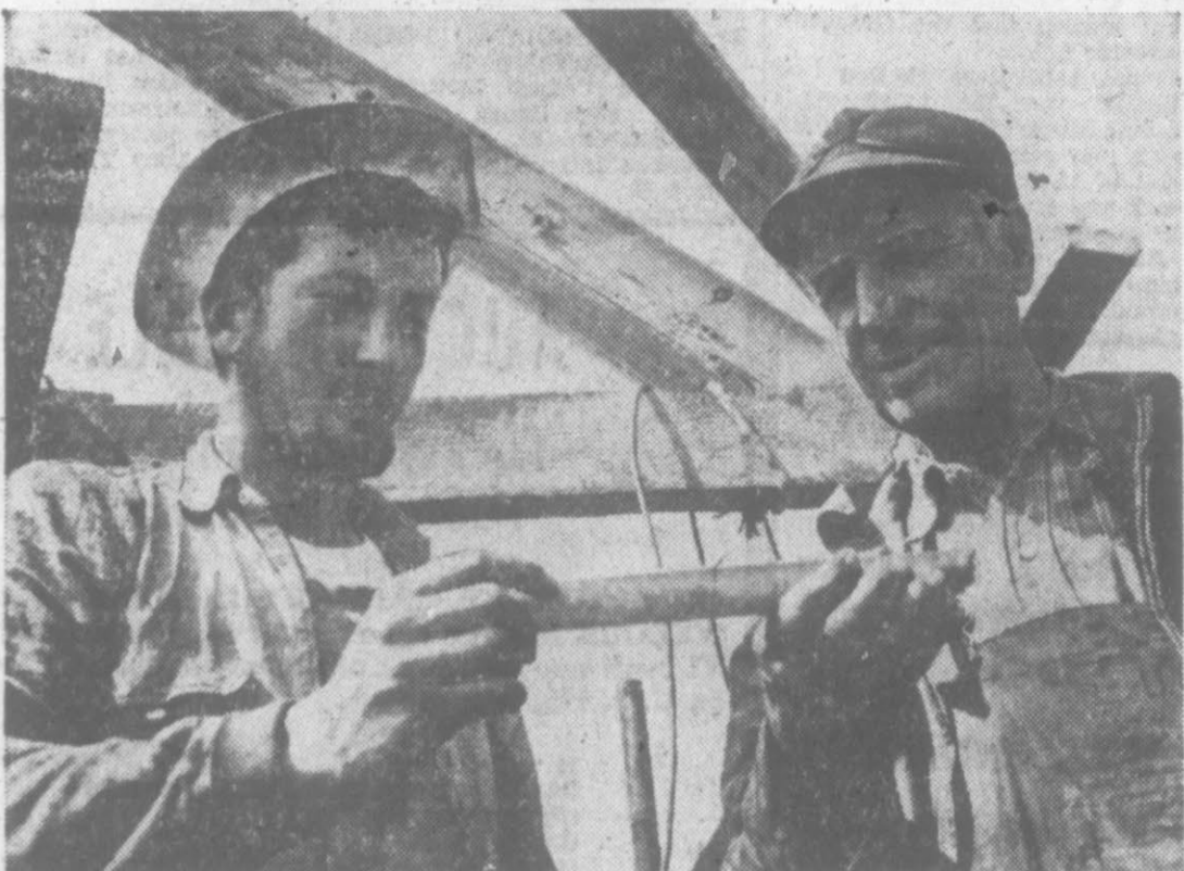
Core of rock, with promising traces of copper, is examined by miners Frank Olander, left, and Harold Everson. Core had been taken from exploratory drill that had penetrated more than 1,000 feet into Miners' Ridge.
