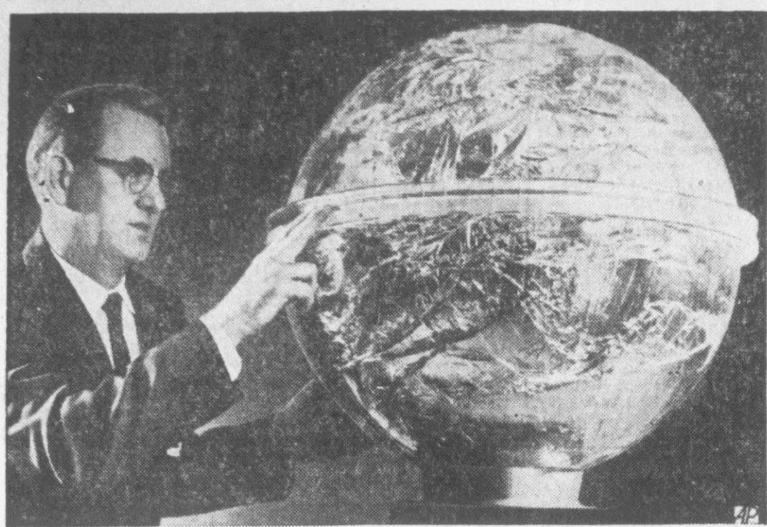
PACKED FOR PROBE — Scientist at Langley Research Center in Virginia examines flight package of a 100-foot sphere, part of the NASA's inflatable satellite program. The sphere, which can be a lunar probe, inflates automatically in space.
