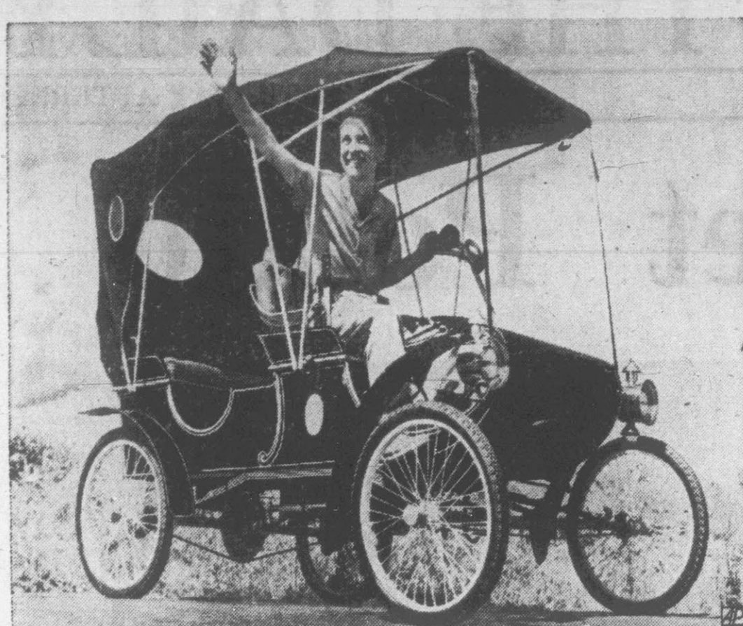
RENEWING OLD TIMER — William Barnhart waves from 1903 Oldsmobile at Waynesboro, Pa. He's in business of duplicating the antique Olds but with modern appurtenances — self-starting 7.95-horsepower engine, automatic transmission and the like.
