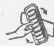
HEAT GUIDING OUTLETS Just pull and turn to guide the Super Floor Heat.
