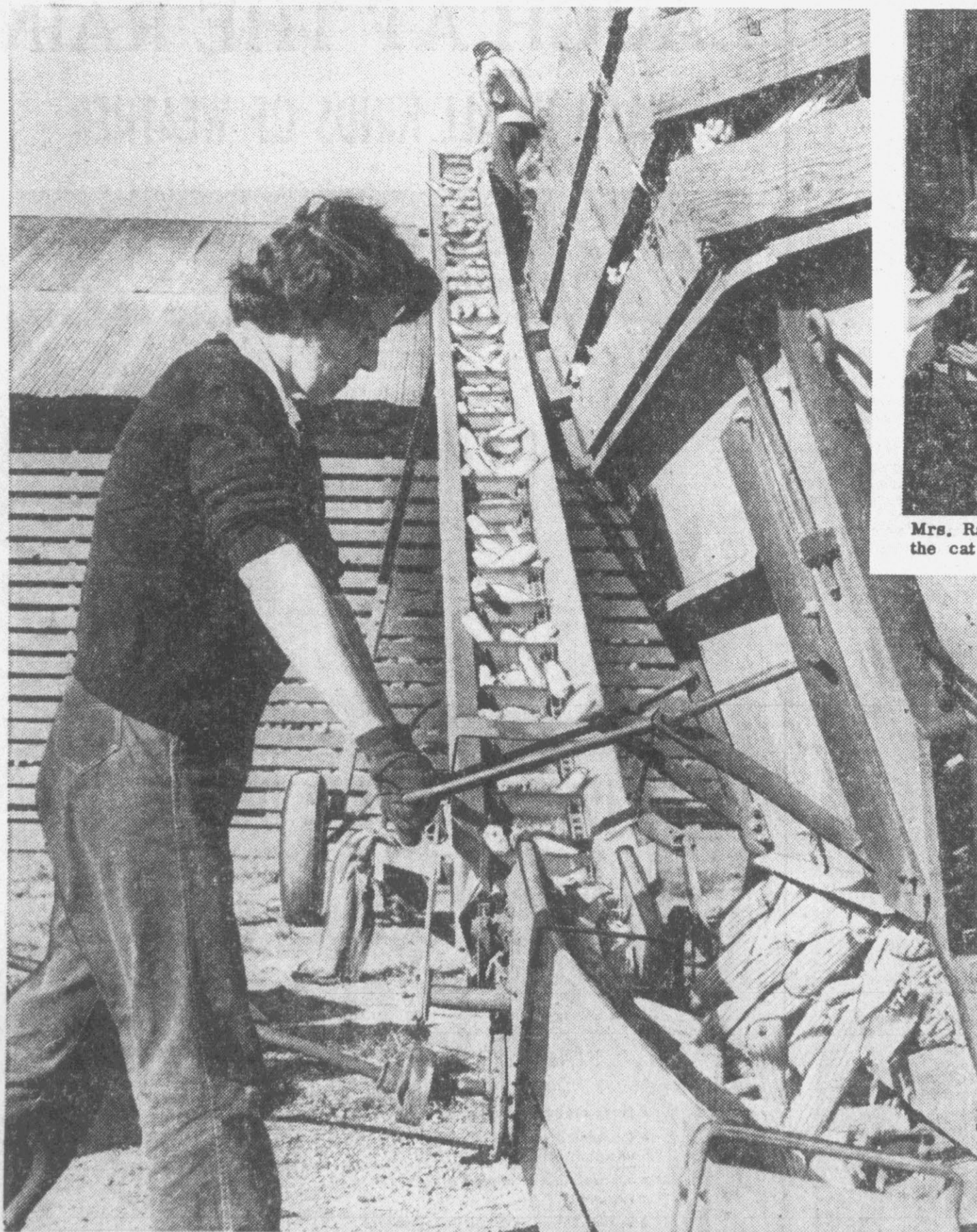
Mrs. Russell Carr dumps corn from a wagon into a hoist which carries it to a crib. She regulates the flow by raising or lowering the endgate to prevent an overflow.
