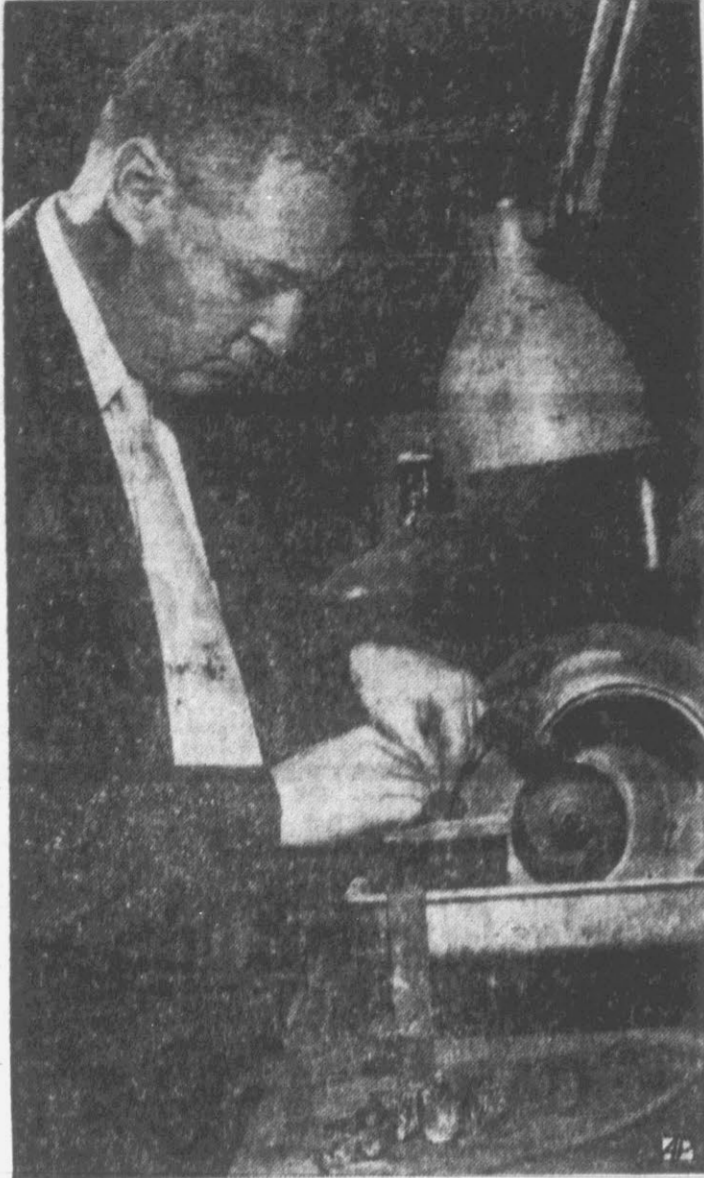
LABORATORY MINER—Carroll F. Chatham cuts a 30-carat emerald with a diamond saw in his San Francisco laboratory. Chatham grows the emeralds himself by a top secret process.
