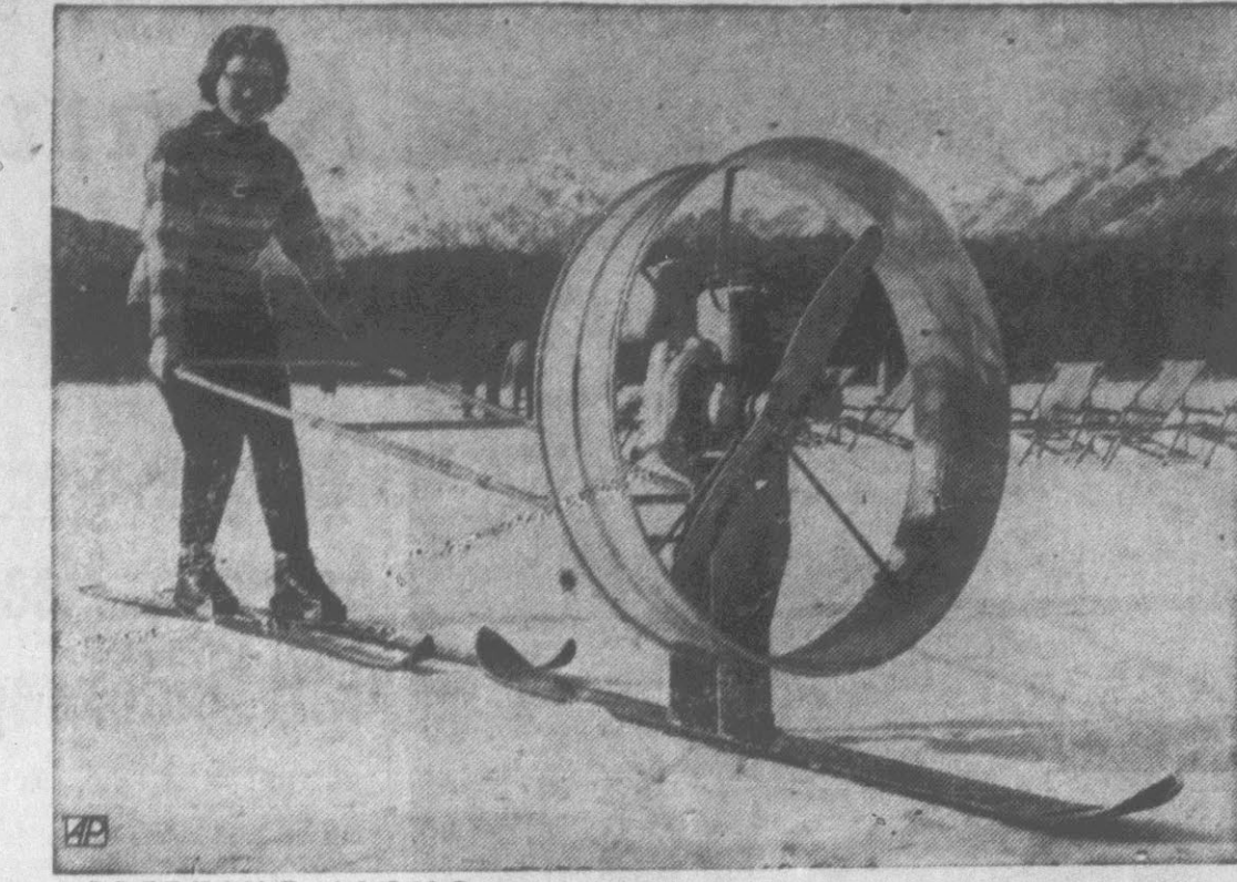
BREEZING ALONG —A ski enthusiast at Garmisch, Germany, tries a "ski pony," a propeller-driven gadget, which can pull skier at speeds up to 30 miles an hour.
