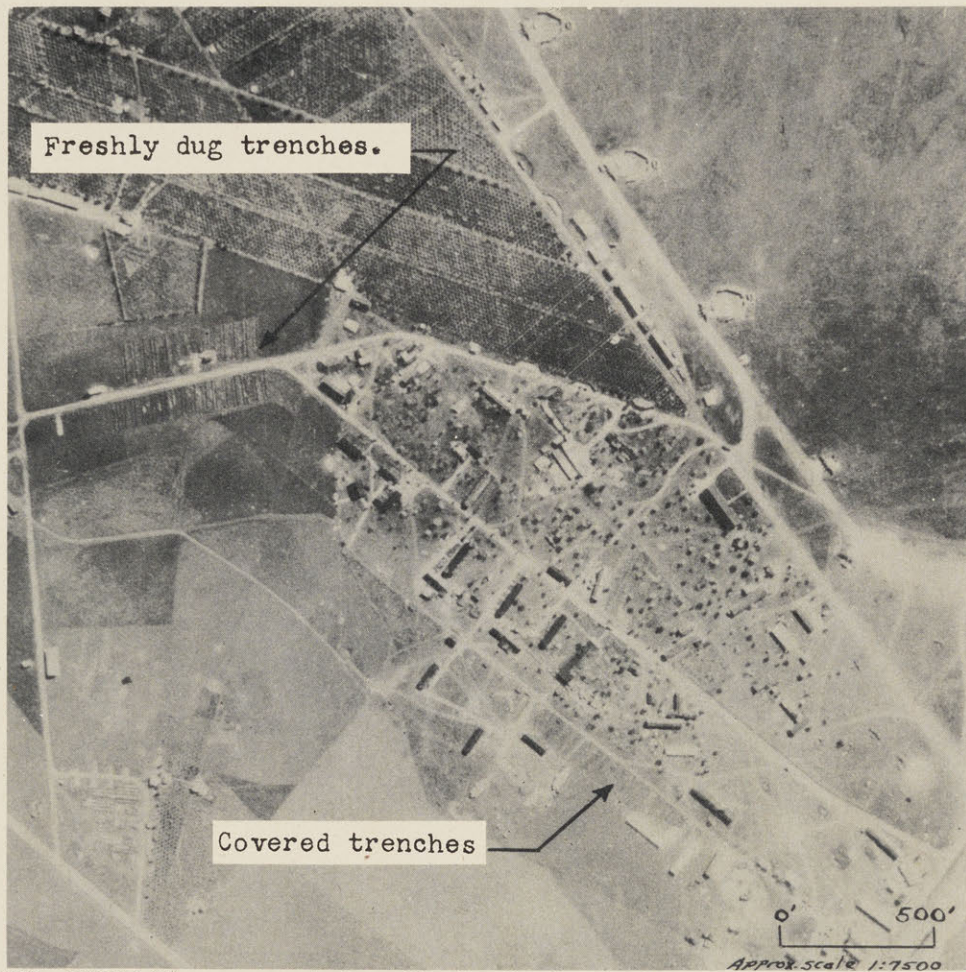
FUEL STORAGE: Suspected method of storing individual cans or barrels of fuel. Similar trenches are seen at Gela and Catania airports.
