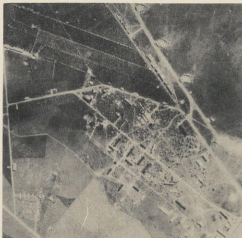
FUEL STORAGE: Suspected method of storing individual cans or barrels of fuel. Similar trenches are seen at Gela and Catania airports.
