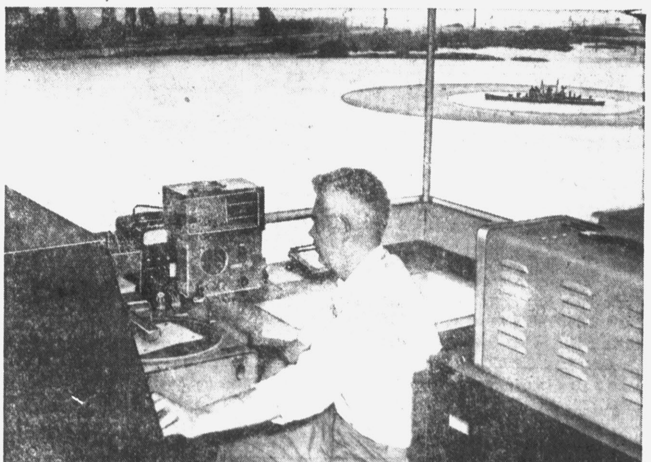
Leo P. Wilbert makes antenna pattern of Boston-class cruiser. Model cruiser on turntable, in distance, is rotating at same speed as turntable in front of Wilbert.
