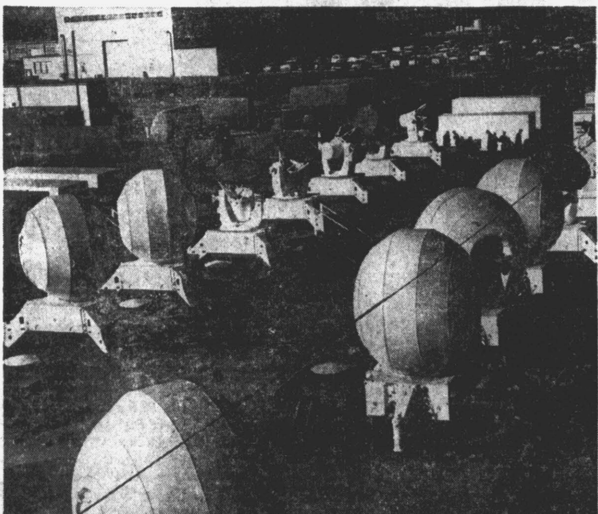
Radar equipment for use by students crowds campus at the missile school. The bulky round mechanisms are used for tracking missiles in flight.
