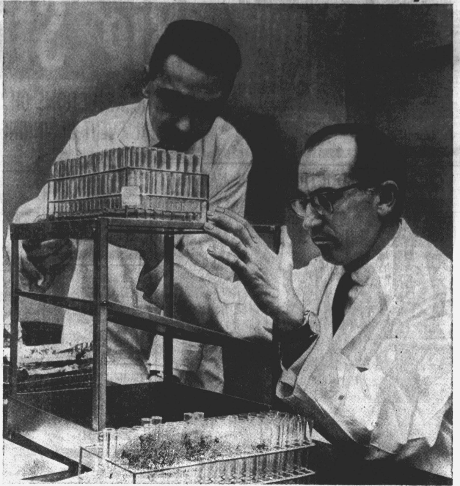
In laboratory room, Salk reads result of tests. Outcome is determined by varying colors of material in tubes, which can be seen in slanted mirror on rack. Research associate Abel Prinzie watches.
