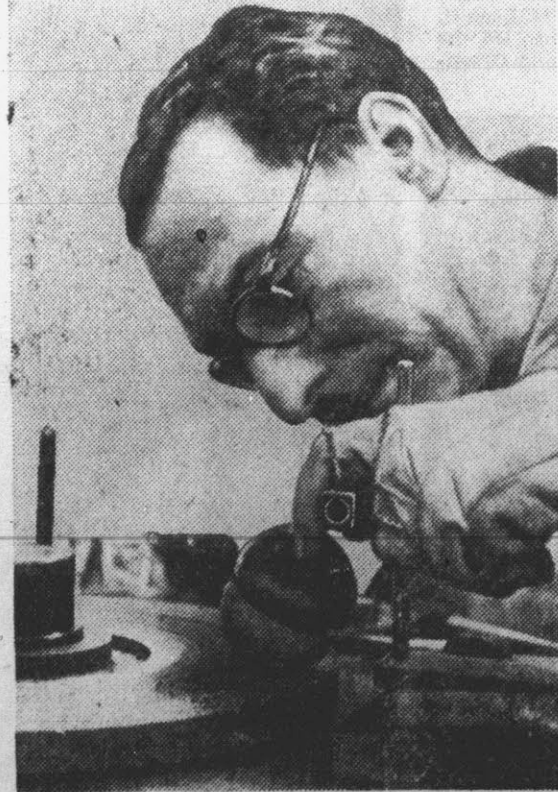
9. Diamond is then mounted in lead dop, or cup, and held close to wheel for final polishing.
