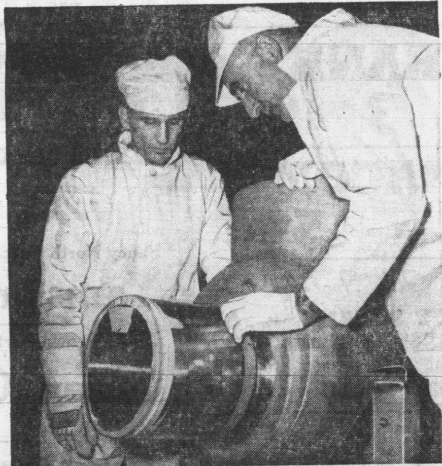
Marvin Gann, welder, and Gerald Inman, inspector, right, assemble component part of submarine inside "surgically clean" assembly tent at Mare Island Navy Yard.
