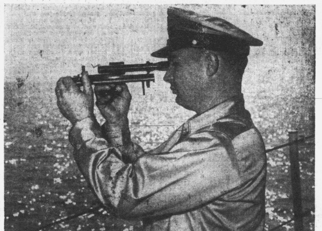
Exact position of the Ambrose, all-important to passing marine navigators, is verified with a sextant. Storms sometime blow the sturdy craft off location in spite of her 7,800-pound steel anchor.
