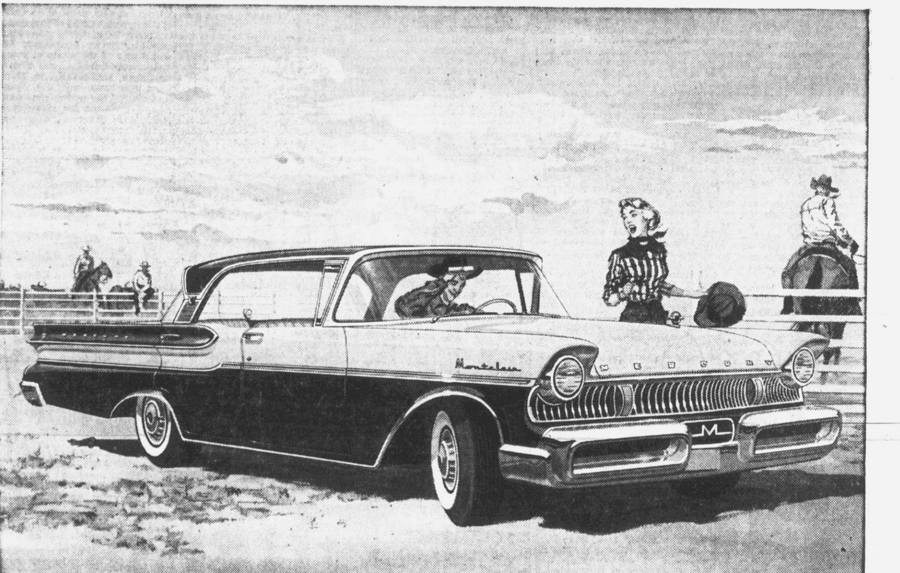
YOU ENJOY INCREASED HEADROOM—made possible by recessing the floor within the frame, and by the unique, straight-line design of the roof. Mercury's outside height is a sleek, shoulder-high 4 feet 8 inches.
