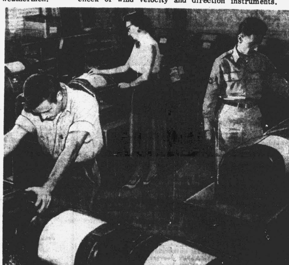
Teleprinters, running continuously, record weather data from all over the world. From this data weather maps and forecasts are made. Operation is staffed by Weather Bureau, Air Force and Navy personnel. This Week's Picture Show by AP Staff Photographer Henry Burroughs
