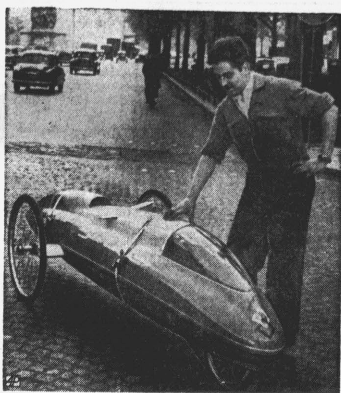
PARISIAN THREE-WHEELER — This three-wheel vehicle, equipped with bicycle wheels and a 49cc motor, is said to have reached a speed of 71 mph in Paris tests.
