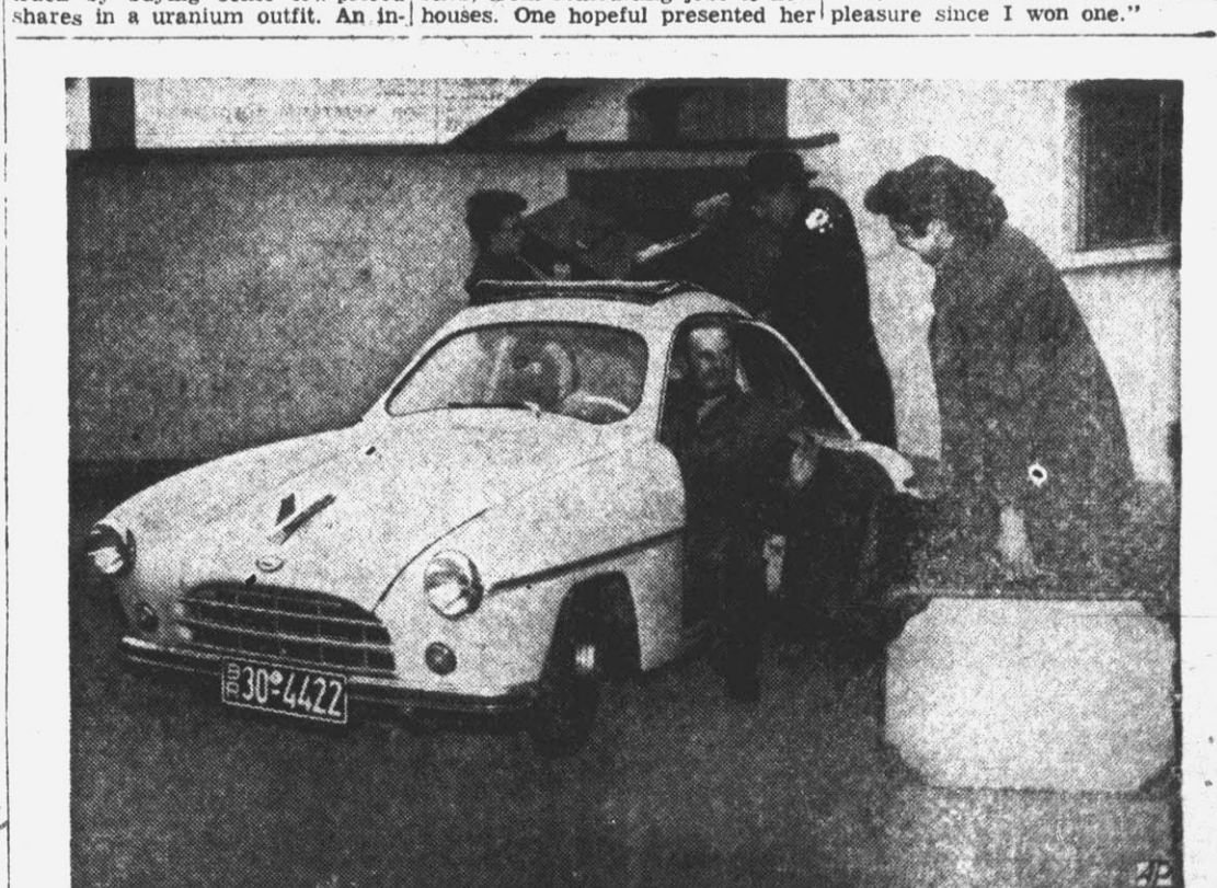
SMALL BUT MIGHTY — Four people and their luggage can fit into this German car, the Kleinschnittger, which weighs only 600 pounds, travels 62 miles an hour and sells for $821.
