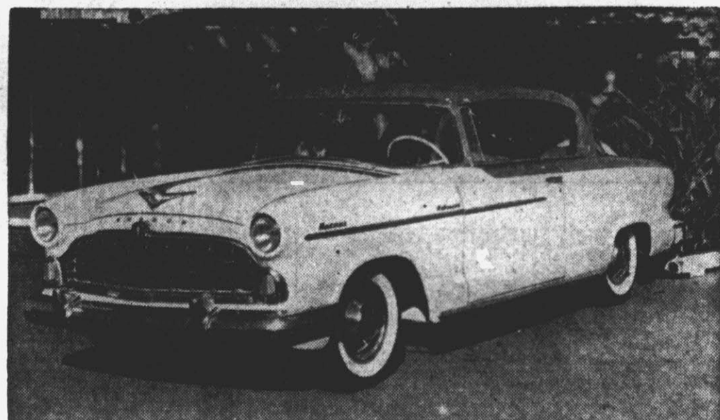
Completely restyled from front to rear, the 1955 Hudson Hornet features sleek body lines, a continental-styled one-piece grille, wrap-around windshield, double strength single unit body, and improved suspension system. A wide choice of high-performance engines are available, including a new V-8 of advanced design. Reclining seats and twin-travel beds are standard on custom models. The industry's most advanced and lowest priced air-conditioning system is available for all '55 Hornet, Wasp and Rambler models.
