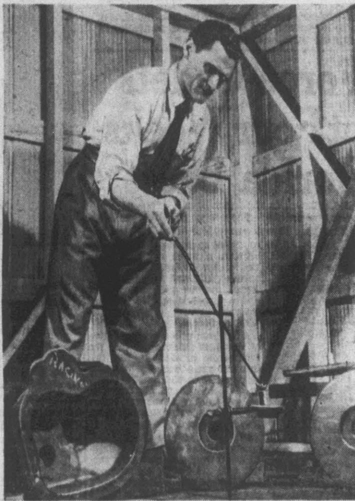
Metallurgist R. Kijowski deposits source of Cobalt-60 in center of ring of castings. Flaws show up on sensitized photographic paper by exposure to radiation.
