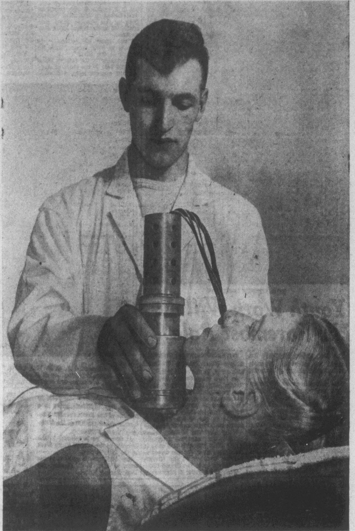
Technician George Serif uses scintillation counter on thyroid patient to trace radioactive iodine which has collected at source of goiter.
