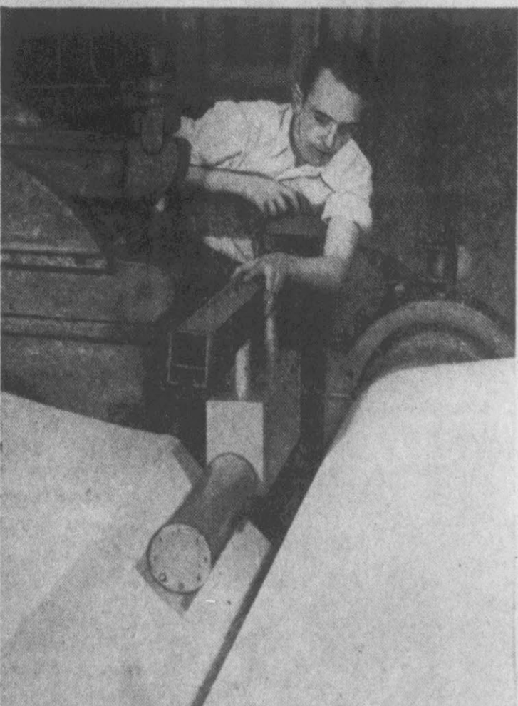
Betameter using thallium isotopes measure weight of paper at Toronto paper plant. The betameter assures uniform weight and thickness by automatic control.
