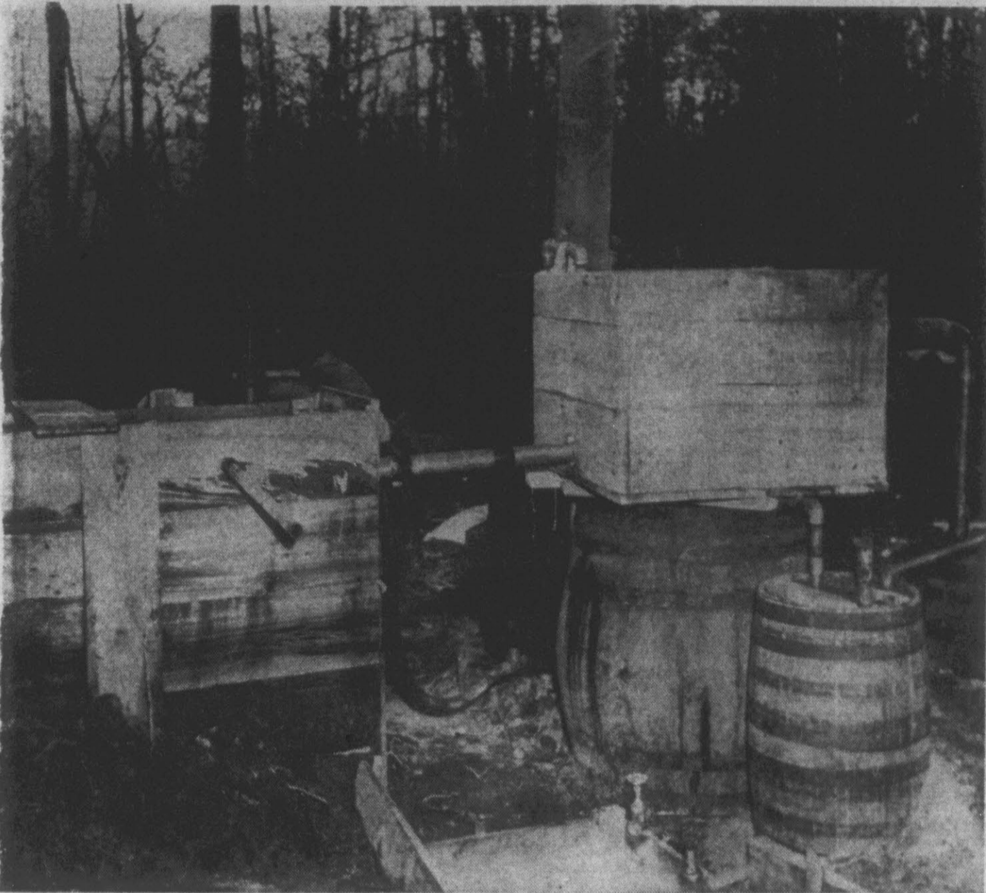
The above photo of a large still found in Pitt County shows the duffers at extreme right which take the water and other impurities out of the distilled liquor. The box above the duffer is the pre-heating unit where the mash to be fed into the still is kept warm. On the left is the cooling unit which contains the condenser for cooling the liquor.
