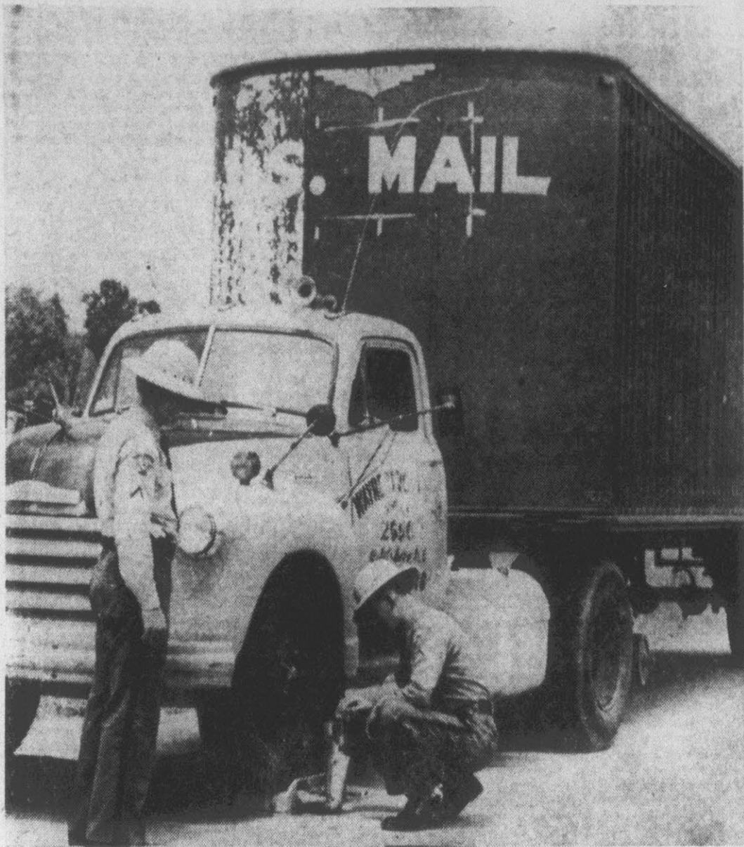
Two local North Carolina Highway Patrolmen are shown here weighing a truck with "portable scales." The truck is being checked to see if it is overloaded. With these portable scales the patrolmen can set up a "weigh station" at almost any point on the highway. This shot was taken on N. C. 11 near Greenville yesterday. The two patrolmen are James W. Boykin, kneeling, and D. E. Perry. (Reflector Staff Photos by Bob Boyette)
