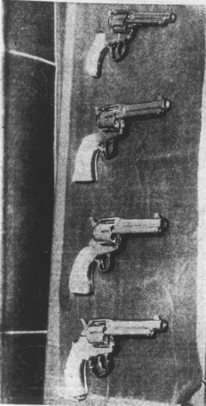
SYMBOLS OF THE ROARING WEST —These four guns represent the most famous firearms ever made by the Colt Company. At top is a .41 calibre Colt, the type gun carried by Billy the Kid Bonney; below it is a single action Colt .45 Lightning 1877 model. The two bottom guns are a pair of Colt Frontier revolvers, a .38-40 calibre patented in 1871, and another Colt .45. The pistols shown at top and bottom in this picture are the Frontier models most sought-after by collectors.
