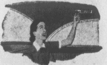
Grilles in Buick's exclusive dual roof ducts insure draft-free distribution of conditioned air—and also provide individual control of air direction as desired.
