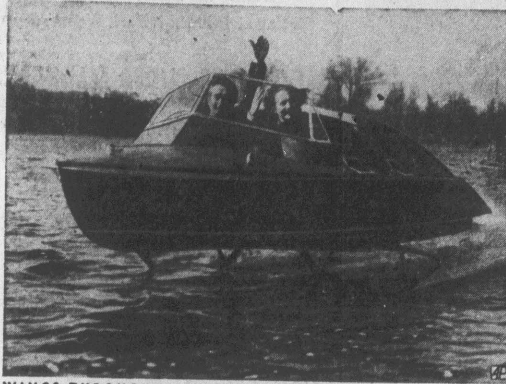
WINGS THROUGH THE WAVES —New German speedboat, with wing-like attachments to stay beneath the hull, speeds along Havel River during trial. Top speed is 62 miles an hour.
