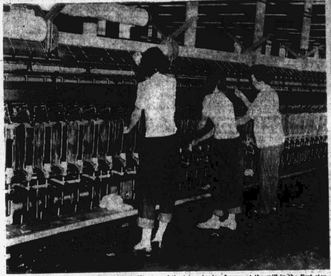
The three women above are setting in operation one of the ten spinning frames at the mill in the first step of spinning the wool into yarn. The roving is taken from the "jack spools" (top), put through the spinning process and becomes yarn.
