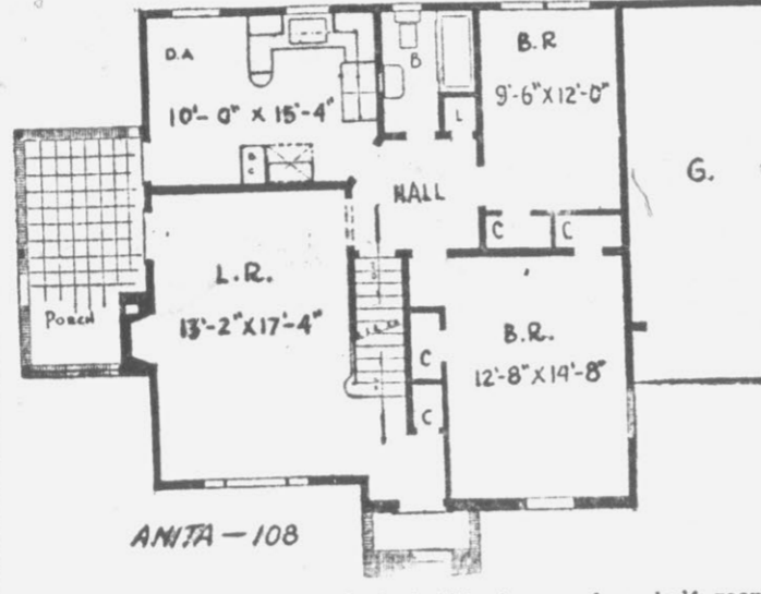
Planned to fit a modest budget, this four-and-a-half room house has an expansive attic where two rooms and bath can be added. Designed by McMurray and Chirgotis, 968 Stuyvesant Avenue, Union, N. J., as the Anita 108, the house covers 957 square feet exclusive of garage and porch. A complete basement is suggested with oil or gas-fired air-conditioned heat.
