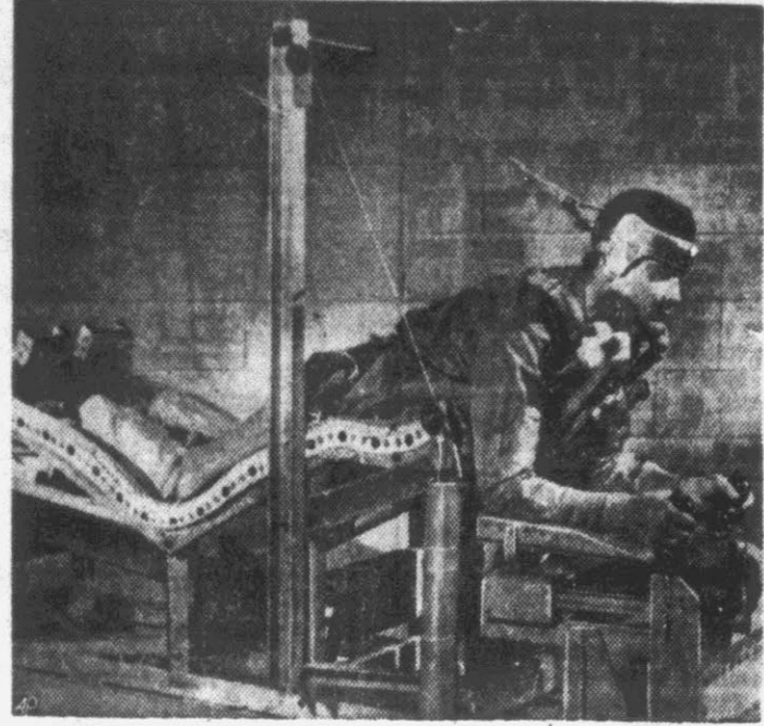
FIRMLY HARNESSSED, the pilot is protected against shock and finds his contoured bed fairly comfortable, while he concentrates on his controls at super speeds.
