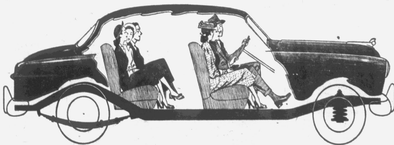
Cutaway views to show the "Mid Ship" Ride and the brand-new springs that let the wheels step over bumps!
