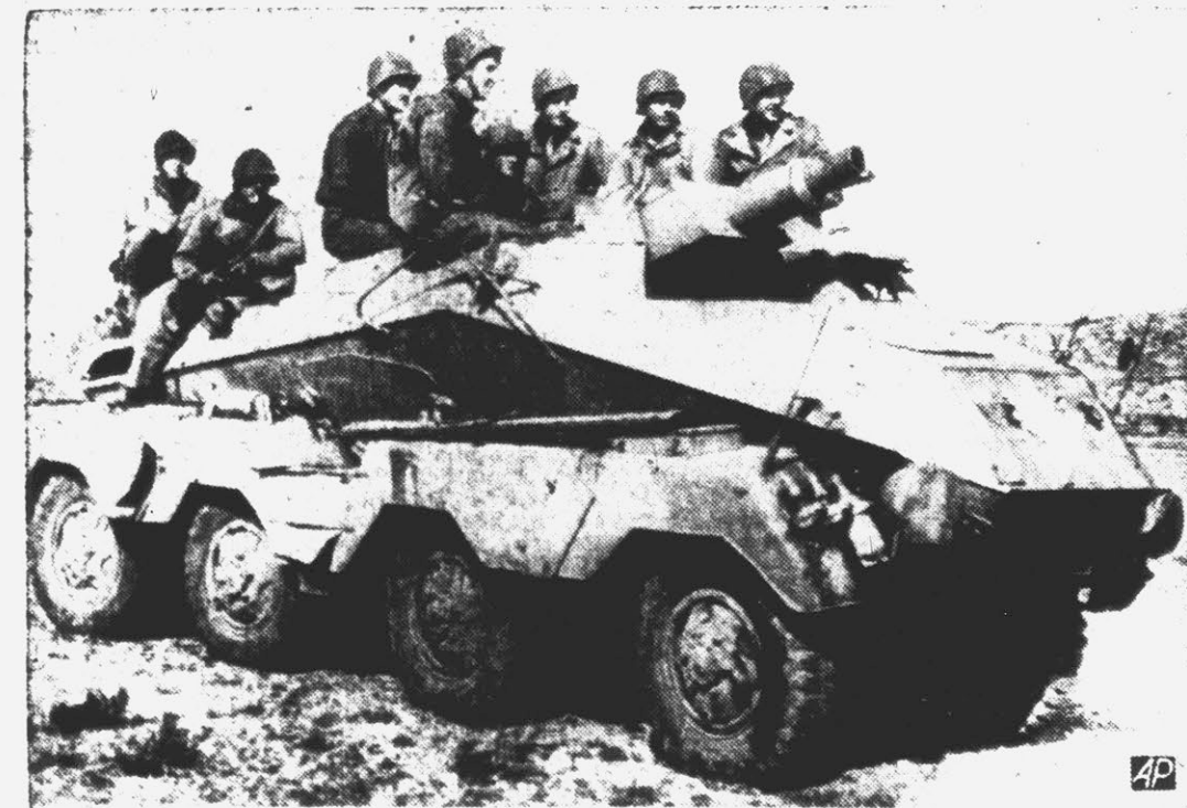
U. S. soldiers ride on a captured German tank destroyer which was taken in a battle with the enemy's 10th Panzer Division in central Tunisia. Equipped with a 75mm. gun and dual controls for operating forwards or backwards, the armored tank buster was used against the Axis after an American star had been painted on its sides.
