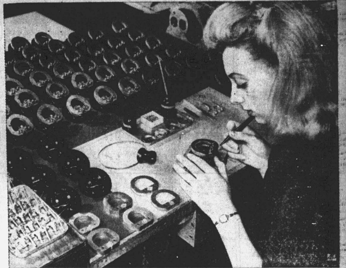
EYES FOR DEFENSE —Like so many eyes looking ahead at the war's outcome are these delicate measuring instruments being assembled at Westinghouse Meter Division. They're destined to serve as mechanical eyes in the cockpits of U.S. army and navy planes. The jeweled instrument movements will go into metal cases and will be equipped with calibrated discs.
