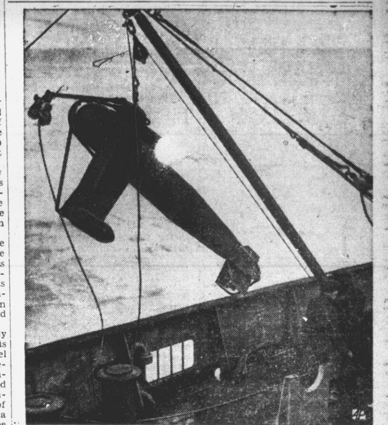
HEADING FOR TROUBLE—Over the side of a British tanker drops a paravane, mine-sweeping device that's towed by ships. A cutting jaw snips anchor chain of the mine which then floats to surface where it's exploded by rifle fire.
