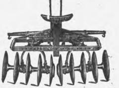
It has a low frame, which will clear overhanging branches and vines. The gange can be set close together or graduated at intervals of two inches until they spread to their extreme width on the ends of the frame.
