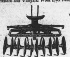
can be set close together or graduated at intervals of two inches until they spread to their extreme width on the ends of the frame.
