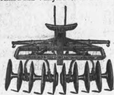
It has a low frame, which will clear overhanging branches and vines. The gangs can be set close together or graduated at intervals of two inches until they spread to their extreme width on the ends of the frame. Two levers-one for each gang-and the gangs can be operated at any angle.
