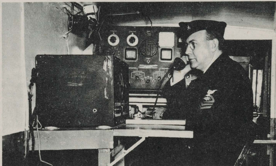
Interior view of Truck, showing on left shelf, Standby Receiver ACR 175, made by R.C.A. In Background, Jefferson-Travis Transceiver, covering from 1,700 KC - 12,000 KC, Crystal Controlled both in Receiver and Transmitter. Charles A. Carter, CRM (T), at the mike.
