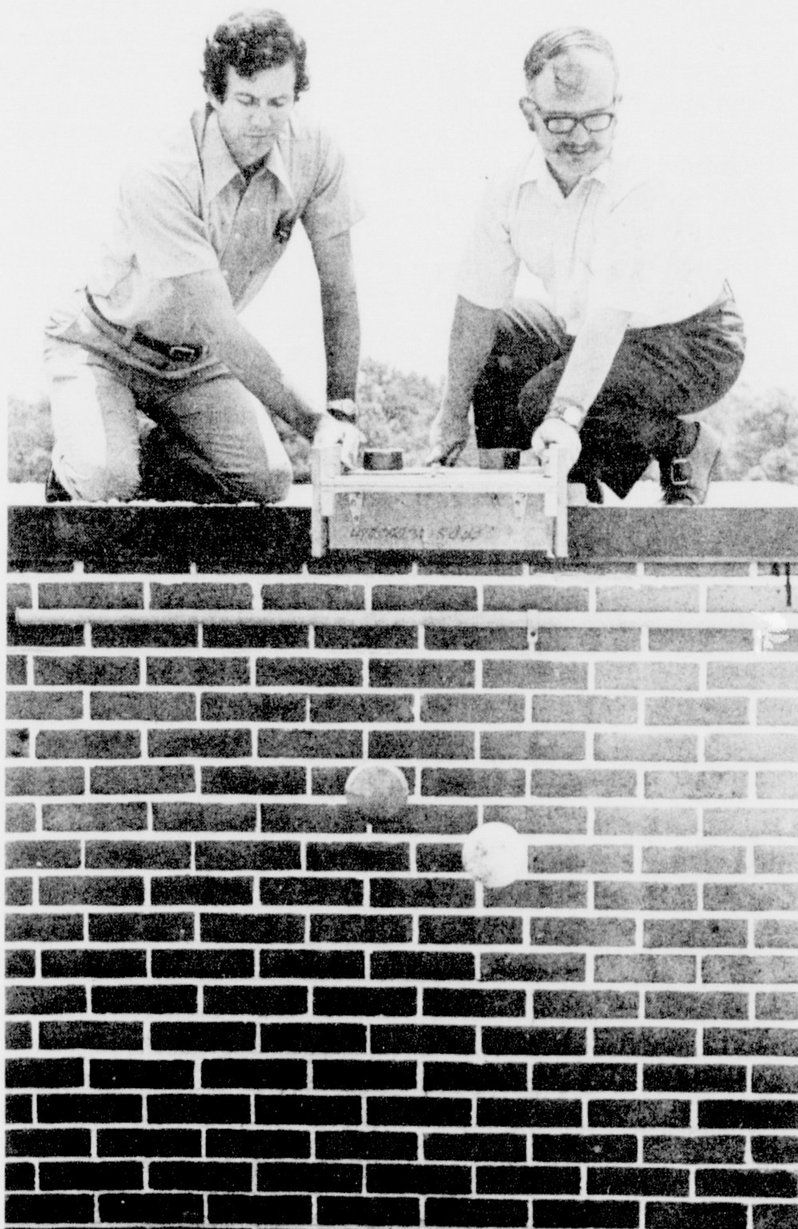
SHOTPUT WINS BALL RACE - Dr. Bryon Coulter and Dr. Carl Adler, East Carolina University physicists, re-enact Galileo's Tower of Pisa experiment by using a shotput, a rubber ball and a specially constructed release gate that enabled them to drop the objects, simultaneously, from the top of an ECU dormitory. The white colored ball on the right is the shotput. [ECU Physics Department photo]
